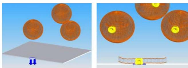
**Figure 1:** The formation of a planar lipid bilayer by vesicle fusion onto a microperforated glass chip is schematically shown.
