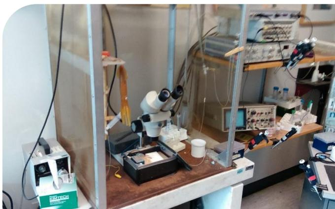
I compare the Orbit mini to our current planar bilayer system, optimized over decades and in daily use here. This consists of a hand-milled plastic chamber consisting of a horizontal partition with a hand-fashioned hole of ~50  $\mu\text{m}$
