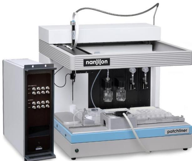
The Patchliner is a fully automated planar patch clamp instrument that records from up to 8 cells simultaneously. With its vast experimental freedom and Giga-Ohm seal data quality, the Patchliner is one of the most versatile patch clamp instruments, predominantly used in cardiac safety studies in the pharmacological industry and in basic ion channel research at Universities and Institutes. The Dynamite<sup>8</sup> is an Add-on of Patchliner.
