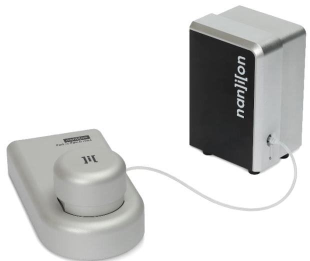
The Port-a-Patch mini is an entry-level patch clamp system, complementing the well-established Port-a-Patch and providing further ease of use, portability and very attractive pricing. However, with its numerous add-ons including external or internal perfusion, temperature controlled recordings, advanced pressure stimulation for mechanosensitive targets or optogenetic approaches, the original Port-a-Patch remains the instrument requiring more complex experimental designs.
