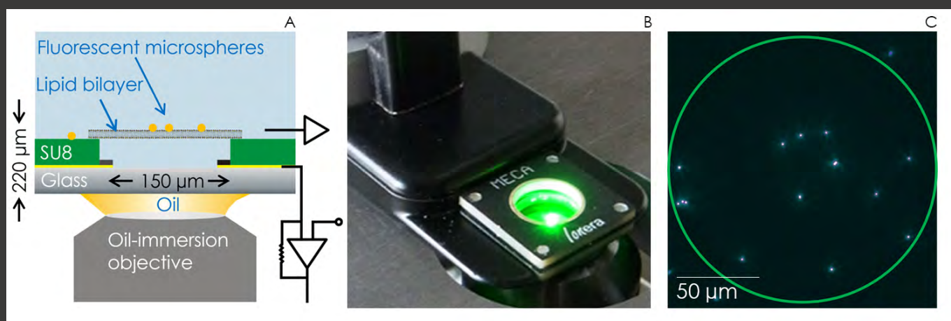
(A) Schematic of the experimental setup for the detection of fluorescent microspheres. (B) The MECA 4 OPTO-INV chip placed above the objective of an inverse microscope. (C) Image of the microspheres on the lipid bilayer - all spheres are in focus.
