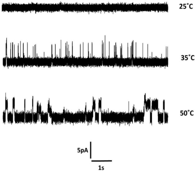
Figure 2. Current traces of reconstituted TRPV1 in DPhPC bilayers recorded at a transmembrane voltage of  $V_m = +50$  mV. The activity of TRPV1 is temperature dependent. The activity of TRPV1 at 3 different temperatures around the activation threshold ( $>42$  °C), 25, 35 and 50 °C is shown. The recordings were done in symmetrical 200 mM KCl, 10 mM HEPES, pH 7.2.
