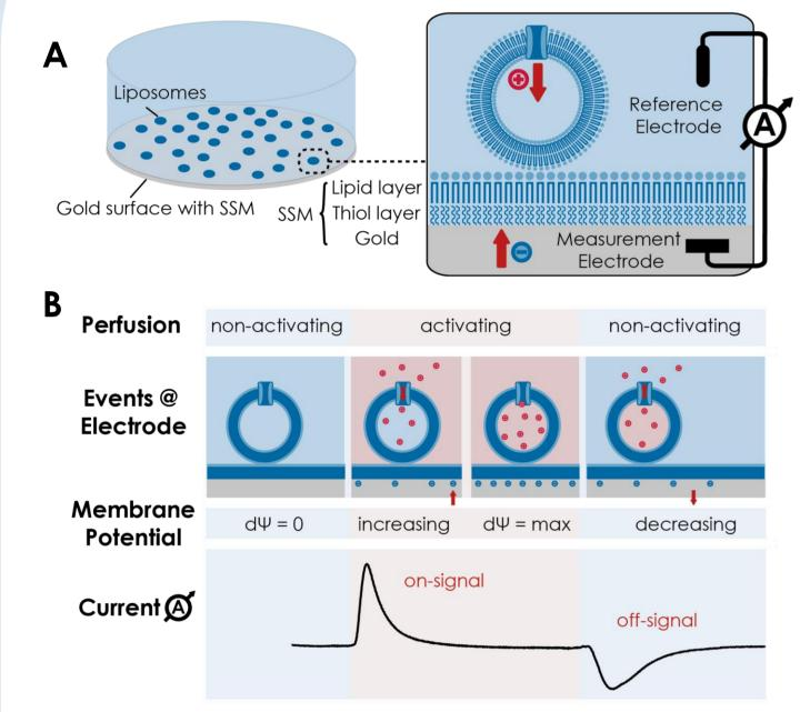
A: Structure of a SSM sensor. The 3 mm diameter thin layer gold electrode is coated with a SSM consisting of a thiol and a lipid monolayer. On top liposomes or membrane vesicles containing the target protein are adsorbed.
