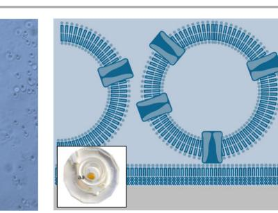
The cardiomyocytes were added to a lipid coated SSM sensor. The sensor was centrifuged to form a tight connection of the cells with the lipid
