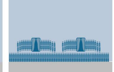
The sensor was rinsed in a fluidic system with high speed. This leads to tearing of the cells - only a membrane sheet remains. This is a hypothesis, investigation is necessary.
