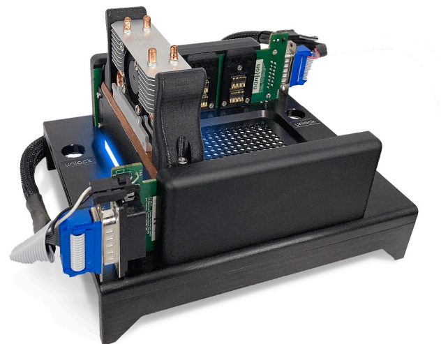
The picture above shows one LED module mounted on the SyncroPatch 384 electrode board.
