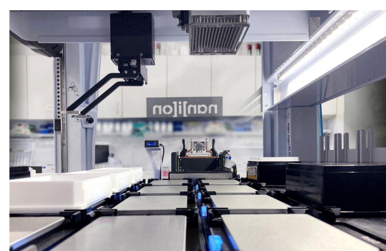
Figure 2: Light activated ion channels can be recorded on the SyncroPatch 384 with Optogenetic Stimulation Tool (above). A ChR2-Na v 1.5 expressed in HEK cells recorded on the SyncroPatch 384 with light stimulation add-on. Whole-cell ChR2 currents were elicited using increasing light intensities under constant 100 ms light exposure. B Action potentials recordings with 500 ms blue light pulse durations. Activation of ChR2 by blue light caused membrane depolarization which in turn activated Na v 1.5. HEK cells expressing ChR-Na v 1.5 were kindly provided by Axxam SpA.
